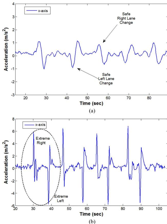
Fig. 7. Lane changes recorded by the  $x$ -axis of a smartphone's accelerometer. A left-lane change is formed by a small decrease, followed by an increase. A right-lane change is formed oppositely. (a) Four safe right-lane changes and three safe left-lane changes in series. (b) Four sudden right and left-lane changes performed in series, totaling eight lane changes.
