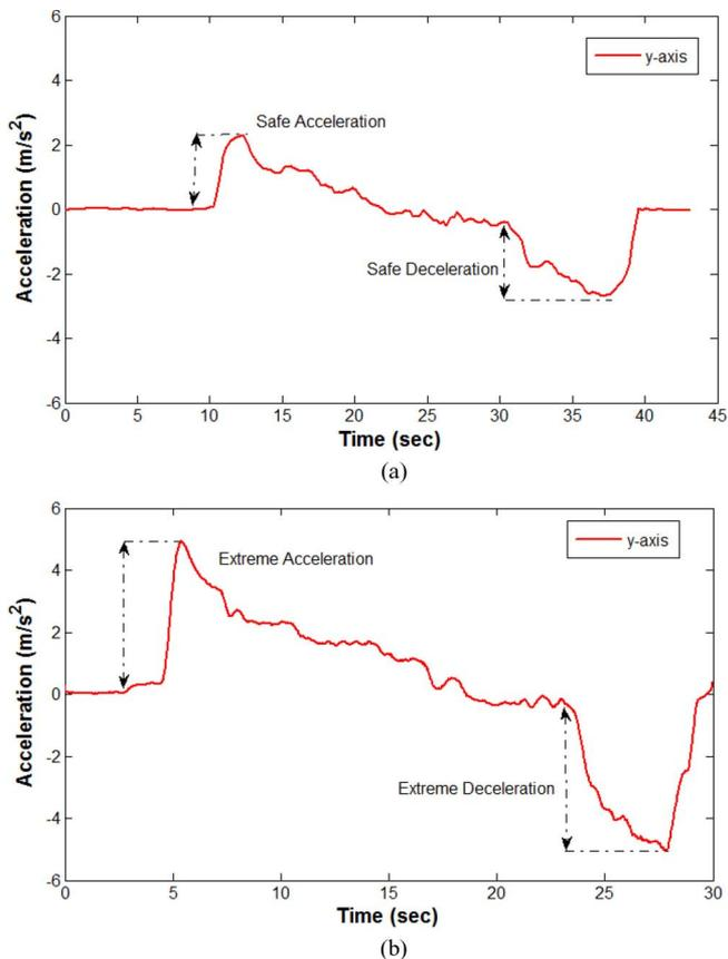
Fig. 5. Acceleration and braking being performed in two different manners. (a) Safe acceleration and deceleration. (b) Sudden acceleration and deceleration. Both are represented by an increase and decrease in the  $y$ -axis, respectively.
