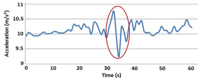
Fig. 9. Speed bump recorded using the  $z$ -axis of the accelerometer at a speed of 7.5 mi/h. This figure correlates with Table IV data, with an originating speed bump height measured at 6 cm.
