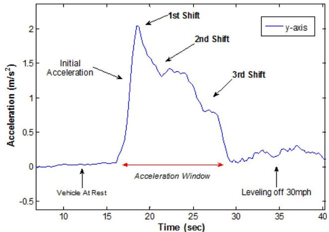
Fig. 4. Engine gear shift analysis of an automobile using the  $y$ -axis of an accelerometer. The vehicle begins at rest, followed by an initial acceleration, with each shift illustrated by a small jerk. The speed at each shift was calculated and compared in Table III.
