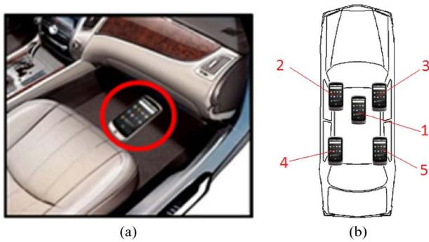
Fig. 3. Phone placement locations in a vehicle. (a) Vehicle floorboard with the  $y$ -axis parallel to the forward motion of the vehicle used for road anomaly identification. (b) Locations in which the phone was tested to measure driving maneuvers. It was determined that loc. 1, which is the center console, gave the best relative data with low engine feedback.
