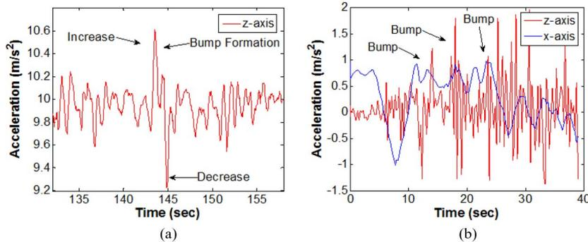
Fig. 8. Bumps recorded using the mobile phone accelerometer. (a) Formation of a bump with an increase in the  $z$ -axis, followed by a decrease. (b) Secondary process in classifying a bump that incorporates the  $x$ -axis. An increase in the  $x$ -axis, followed by the identification method in (a), helps distinguish a pothole from a bump.
